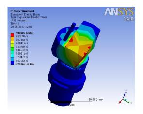
Figure 7: Strain distribution in fixture.
