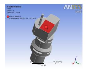
Fig 4force on fixture
