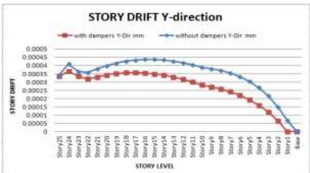
Graph 7: Storey drift in Y direction for Static method
