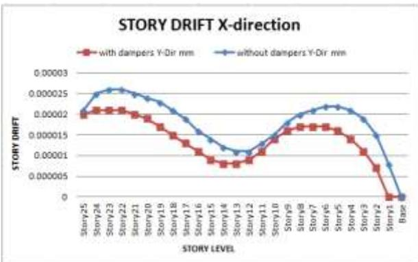
Graph 6: Storey drift in x direction for response spectrum method
