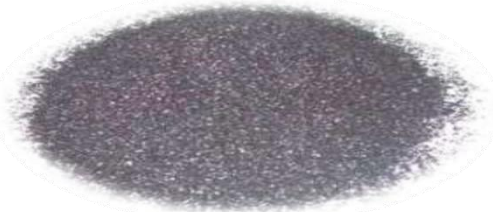
Fig 3.1 Image of copper slag used in the concrete
