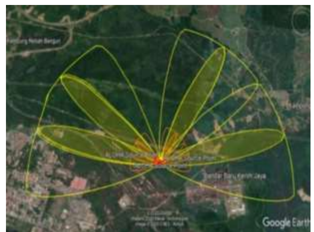
Fig. 5- Area affected from 150 mm diameter leakage (absorber tower)
