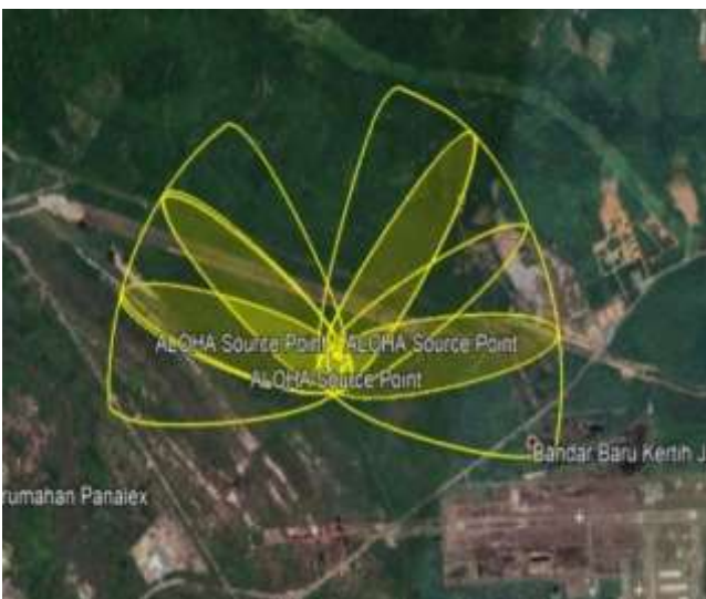
Fig. 4: Area affected from 150 mm diameter leakage (multibed reactor)
