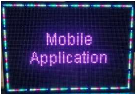
Fig.6 Smart Notice Board Output through Mobile Application using Wi-Fi
