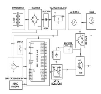
A soft start control technique for the single-phase AC induction motor. It presents a design of a low-cost; high-
