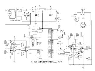
The IGBT is the main control switch here. While drive is given to the G (gate) of the IGBT, the C & E (collector & emitter) closes like a switch thus the ac power flows through the lamp. Thus if the IGBT is triggered with a
