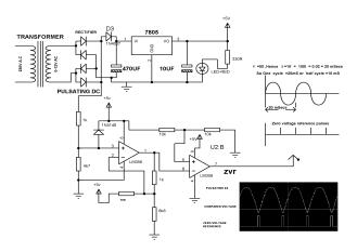
A zero crossing detector is a comparator with the reference level set at zero. It is used for detecting the zero crossings of AC signals. It can be made from an amplifier with an input voltage at its positive input. When the input voltage is positive, the output voltage is a positive value, when the input voltage is negative, the output voltage is a negative value. The magnitude of the output voltage is a property of the operational amplifier and its power supply.
