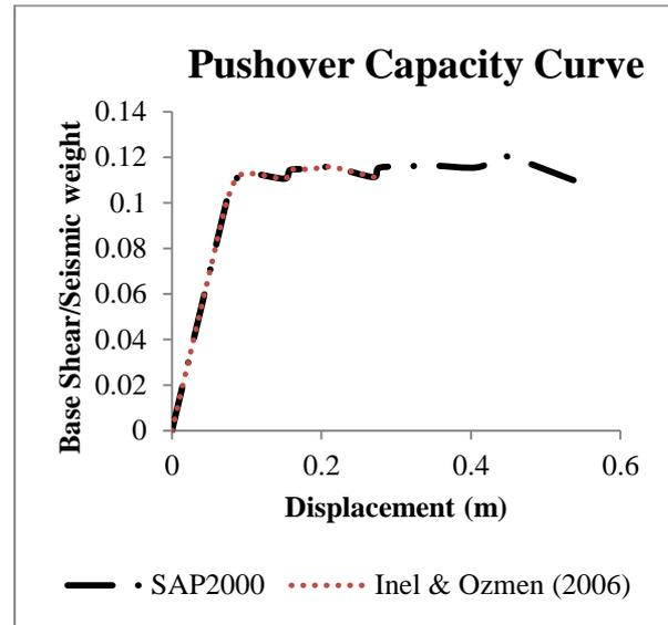
Fig. 2 Validation curve for Pushover analysis
