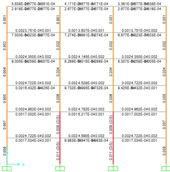
Fig 5. Frame at Y=5 along X-Z direction
