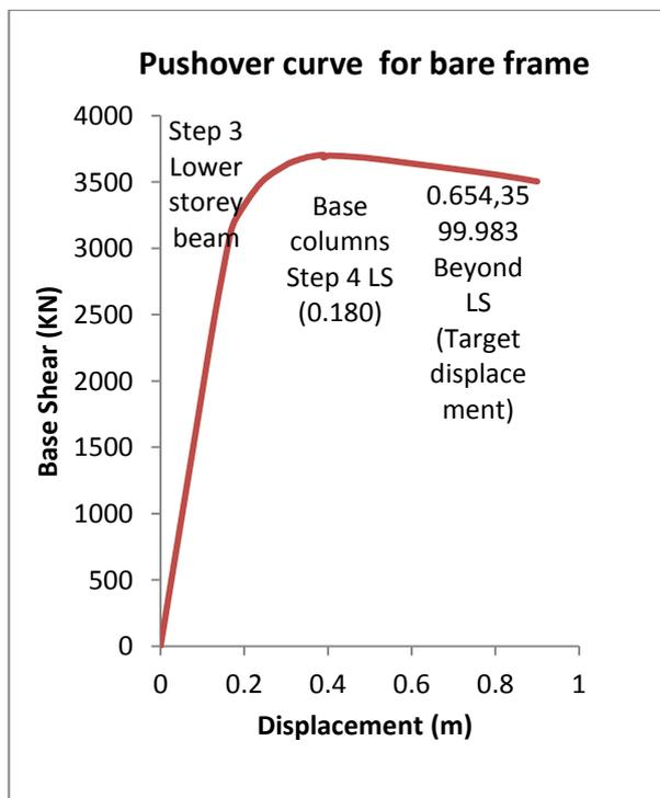
Fig.6 Pushover curve for bare curve
