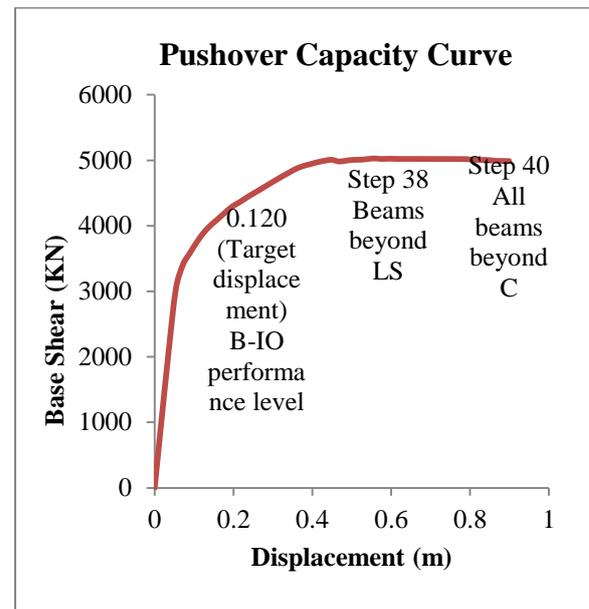
Fig Pushover curve for model with Jacketed elements
