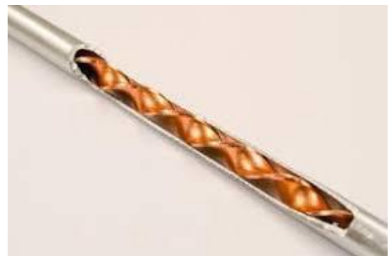
Fig. 3.4 Actual image of Plain twisted tape inserted in tube.
