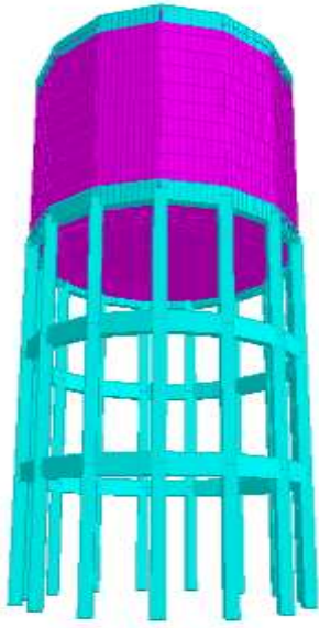
Fig.4 – 3D model of generated water tanks
