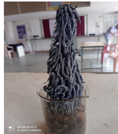
Fig.1 - Synthesized fluffy powder of cobalt ferrite
