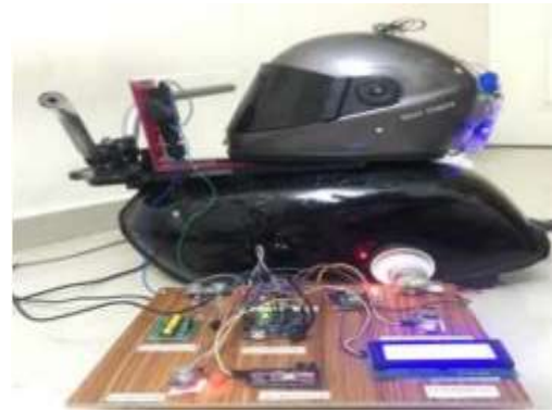
Fig 2. Photograph of the electronic Helmet lock after complete Installation
