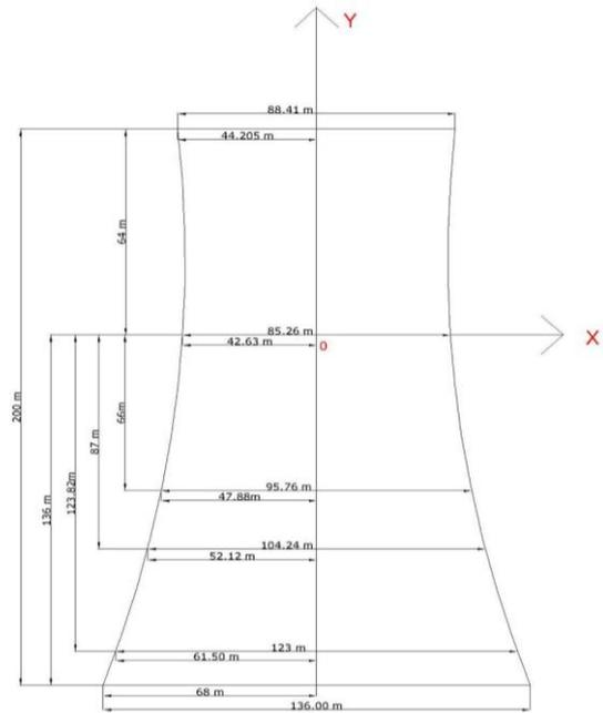
Fig. 1 -Drawing of cooling tower for 68%
