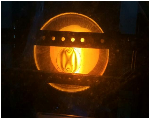
Fig 8-. Fringes developed in calibration disc, loaded under diametric compression
