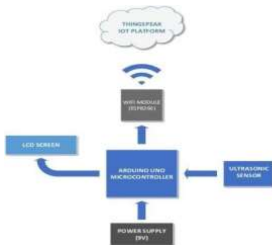
Fig.3. (a) Block diagram for smart waste management system.
