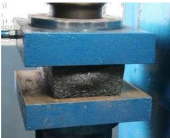
The UTM was using the tests. The compressive strength of bricks. After the curing period gets over bricks are kept for testing. To test the specimens, the bricks are placed in the calibrated compression testing machine of capacity 3000 KN (Kilo Newton) and applied a load uniform at the rate of 2.9 kN/min. By obtaining the maximum load shall be taken as failure of load with specimen fails to produce any further increase in indicator reading on testing machine.
