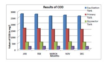
The effluent after force circulation evaporator is treated with Activated sludge process for further reduction in Parameters to achieve permissible limits as per CPCB. In this process, in primary treatment, 40-42 % reduction of COD is observed whereas in secondary treatment 62-65 % reduction in COD is observed and tertiary treatment with 58-60 % reduction in COD. The permissible limit for disposal for COD is 250 mg/l.
