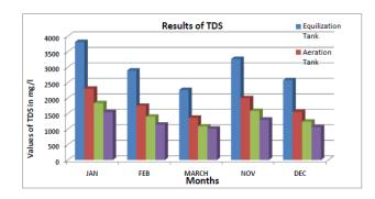
The effluent after force circulation evaporator is treated with Activated sludge process for further reduction in Parameters to achieve permissible limits as per CPCB. In this process, in primary treatment, 38-42 % reduction of TDS is observed whereas in secondary treatment 18-22% reduction in TDS is observed. The permissible limit for disposal for TDS is 2100 mg/l.
