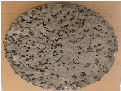
Fig. 1.1- Permeable Concrete Block (Circular)
