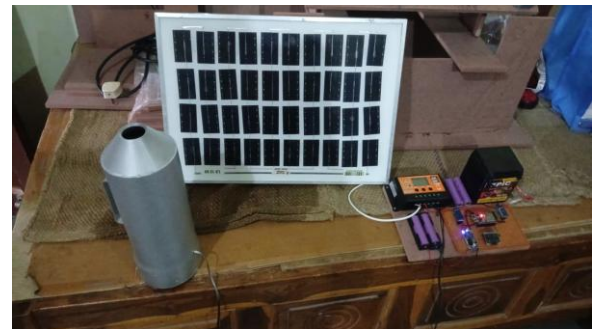
Fig. 3. Assembled prototype of the solar-powered portable dust air blower, showing the solar panel, charge controller, battery pack, Arduino control board and the blower/nozzle unit
